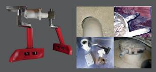
Torsion spring-loaded mixing arm for the retooling of pan mixers
