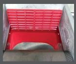
Deflectors for transfer points with pocket buffer, for a grain size from 0 to 32 mm or with step profile, for a grain size from 0 to 75 mm, depending on the profile of requirements.
