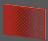
PUCEST® wear plates with a perforated sheet insert were developed as wear protection system for the lining of containers and funnels. The plates are screwed and can be easily installed independently as they can simply be fastened, cut, drilled and bent due to the cast-in perforated sheet.
