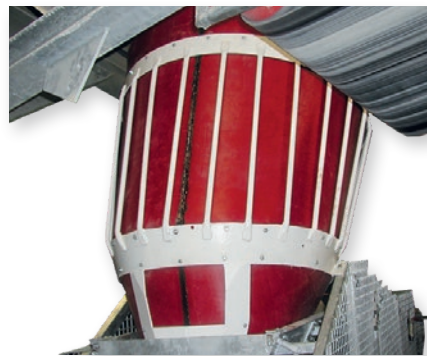
▲ PUCEST ® collection funnel at a belt transfer point
