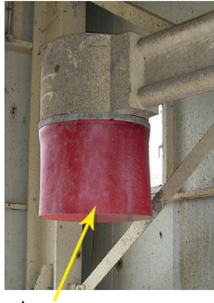
▲ A PUCEST® discharge hose: At this mixing plant a PUCEST® discharge hose was installed at the swivel arm for “self-collectors”.
