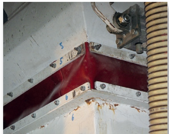
transfer sleeve aggregate scale / mixer
