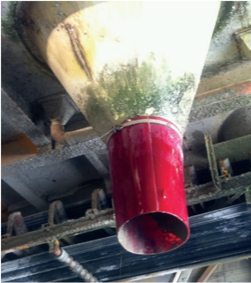
▲ A PUCEST® discharge hose after a wear life span of 100,000 m 3
